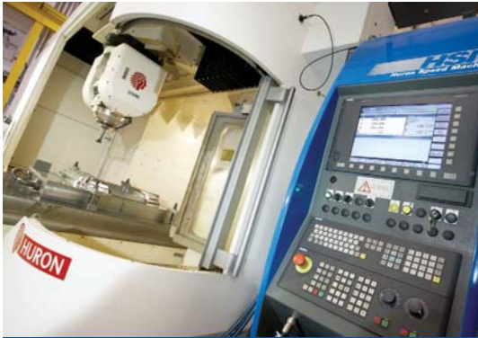
The Huron KX 200 at Delcam's Birmingham headquarters was used to manufacture demonstration parts and the initial production samples.
